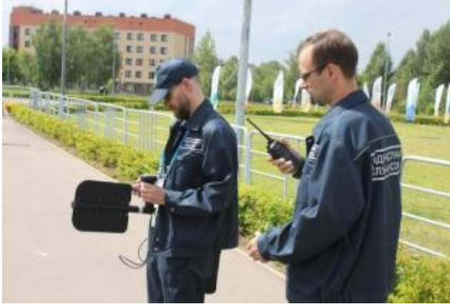
Figure 17. Radio monitoring group during search of an interference source in a stadium
