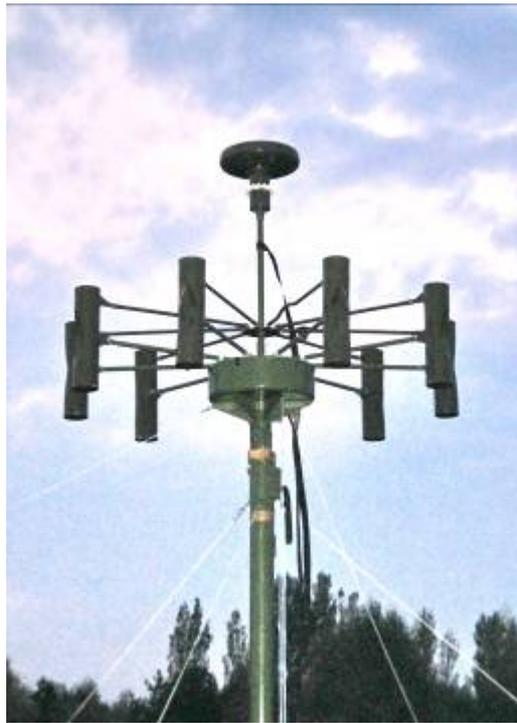
Figure (3). Stationary antenna system with the built-in IF converter for the frequency range 25 - 3000 MHz
