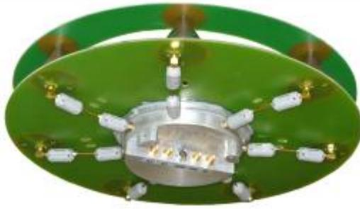
Figure (1). Antenna array with the built-in IF converter for the frequency range 1000 - 3000 MHz
