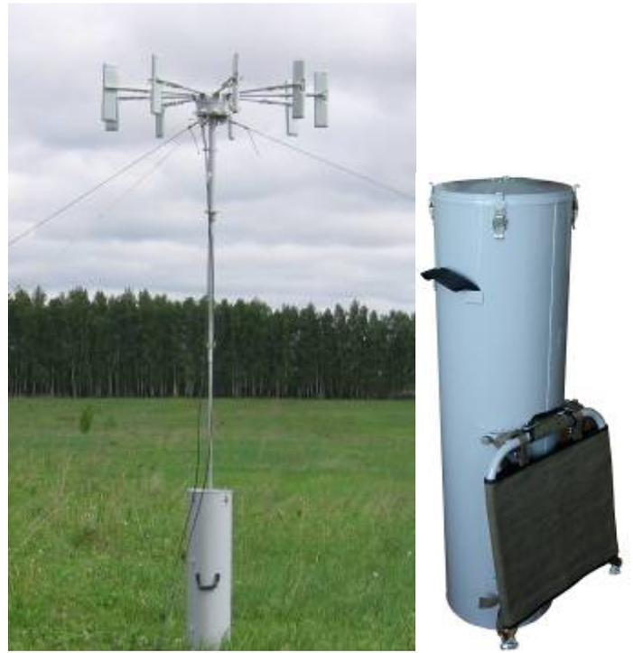
Figure (4). Portable antenna system with the built-in IF converter for the frequency range 25 - 1000 MHz and a case for carrying all antenna components
